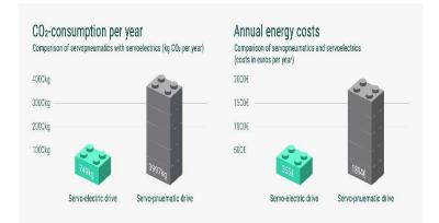
Servo-electric drive saves 4/5 of the energy costs compared to the pneumatic drive – the servo-electric drive can reduce 80% of the  $CO_2$  output
