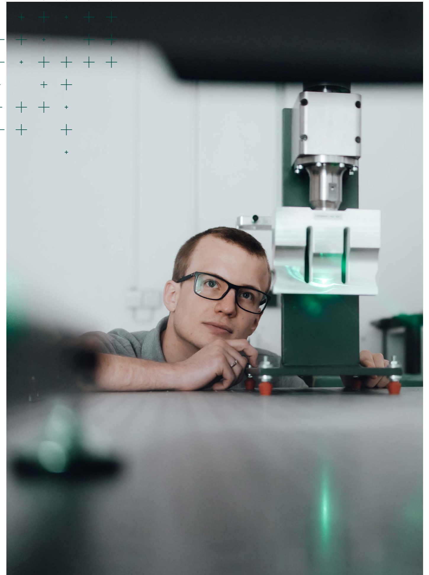
The laser vibrometer provides precise information about the speed and amplitude of vibrations.
